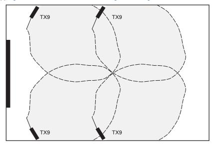
Fig. 8a above is a typical example of how multiple emitters are used to cover larger listening areas. Generally it is desirable for the illumination patterns to overlap. Note: The coverage area will vary depending on the infrared receiver being used; refer to Figures 4 and 7 to determine how many emitters are required to achieve full coverage of a listening area.
